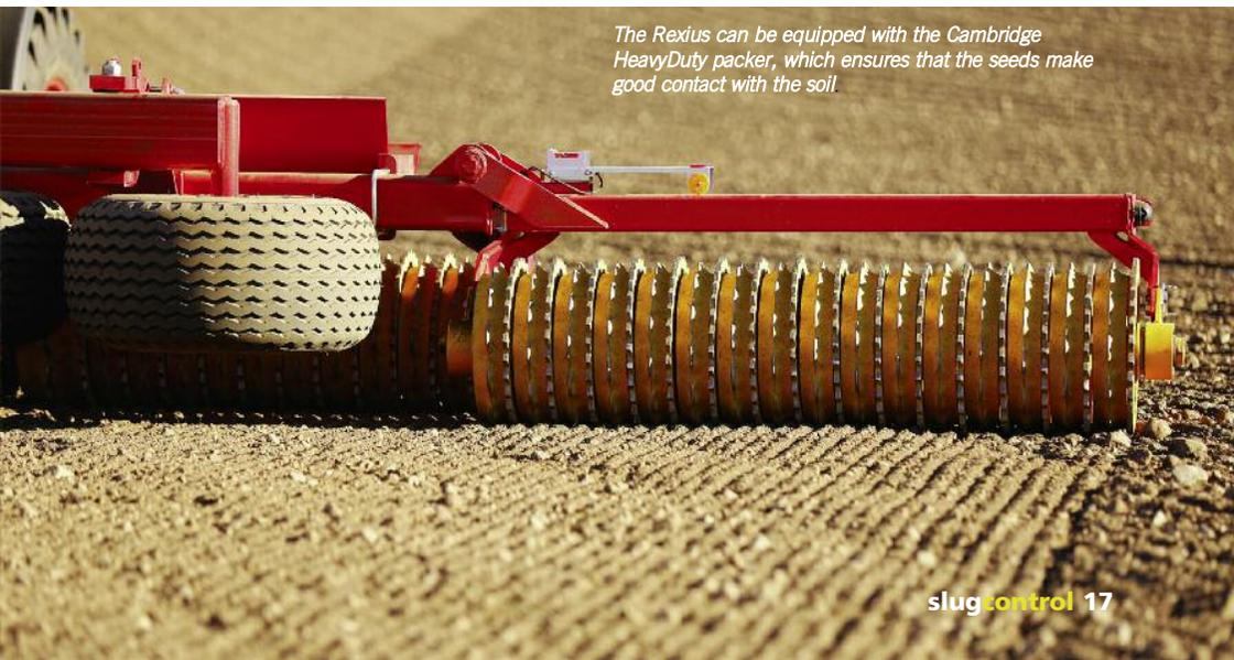
*The Rexius can be equipped with the Cambridge HeavyDuty packer, which ensures that the seeds make good contact with the soil.*
