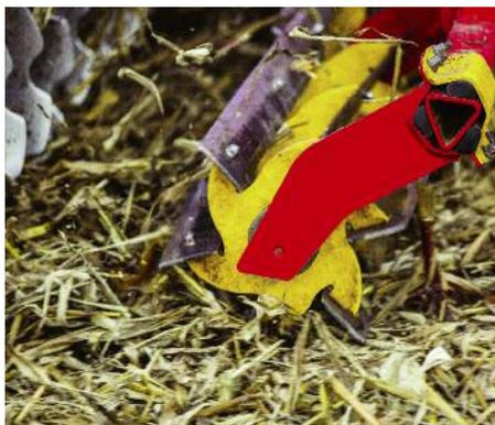
*The CrossCutter Knife is an appropriate tool for destroying stubbles.*
