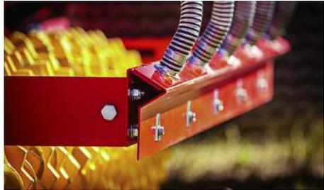
*The design of the spreader plate ensures a precise and even distribution over the entire working width of the machine.*
